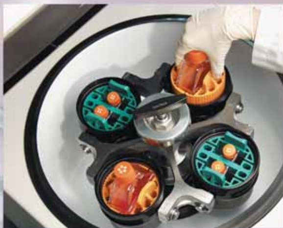
Easily load the adapter into the bucket by grasping the adapter finger grips. Align the narrow sides of the flask to the bucket engraving and the wide sides parallel to the bucket pin pockets.
