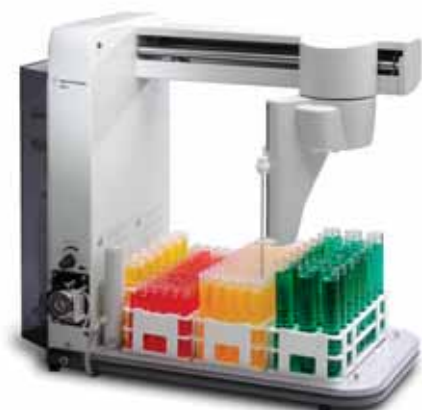
Combine the SVS 1 with Agilent's SPS 3, the fastest spectroscopy autosampler, for up to 30 % improvement in productivity.
